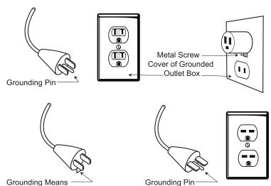
**WARNING**: It is normal for the power cord to feel warm to the touch. However, a loose fit between the outlet and the plug may cause overheating of the plug. If this occurs, try inserting the plug into a different outlet. Contact a qualified electrician to inspect the original outlet for damage.
